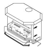
To adjust the aeration: use the allen key to turn the turning gear which will adjust the air shutter. Open the air shutter for a blue flame or close it for a yellower flame. The factory setting should be sufficient for most installations.
